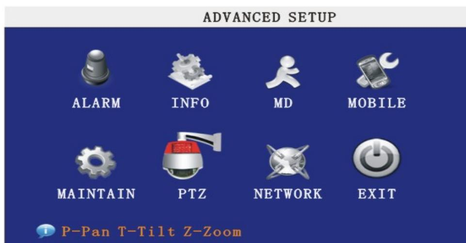
Advanced Features include Alarm settings, system information, Motion detection, mobile phone monitoring, system maintenance, PTZ and network setting.
