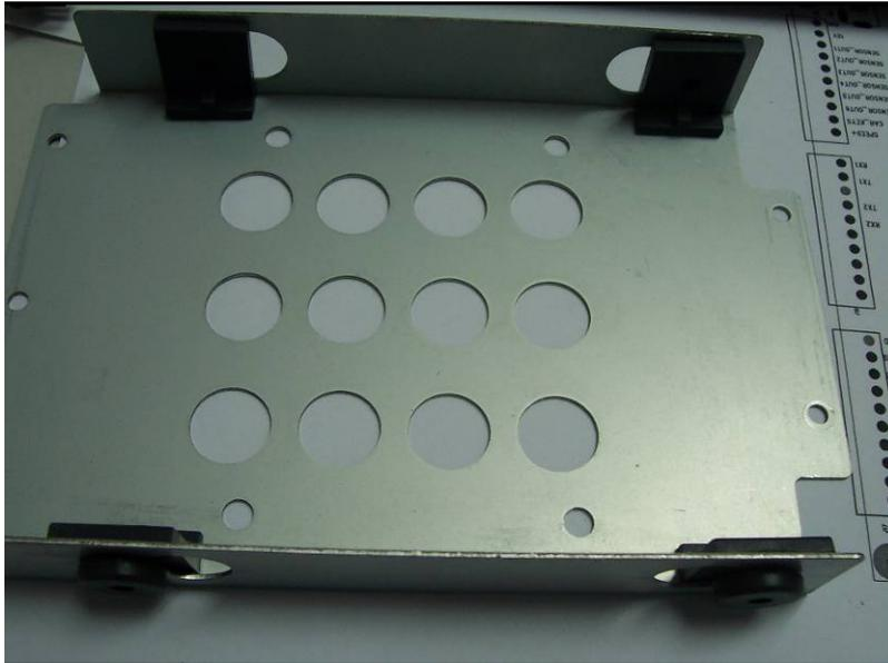
4) Install the HDD on HDD plate as the following photo indicate and then screws around.
