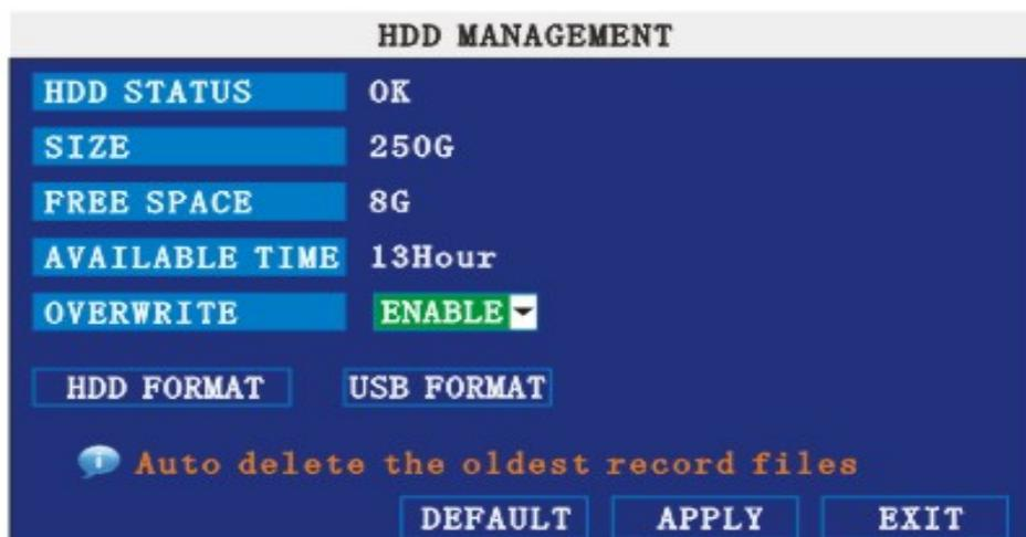
**HDD STATUS:** There are three status available, normal, un-format, No HDD. If HDD can not run normally (including unformat and no HDD) , there is a **【H】** display on video live view.
