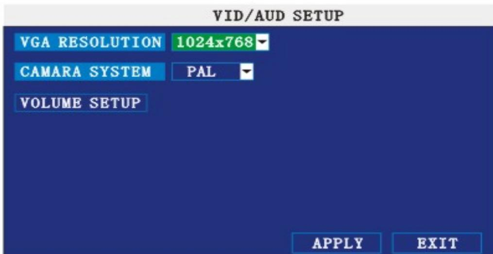
**VGA RESOLUTION:** press **【Enter】** key to setup the VGA resolution, there are 1024\*768、800\*600 and 600\*480 three options.
