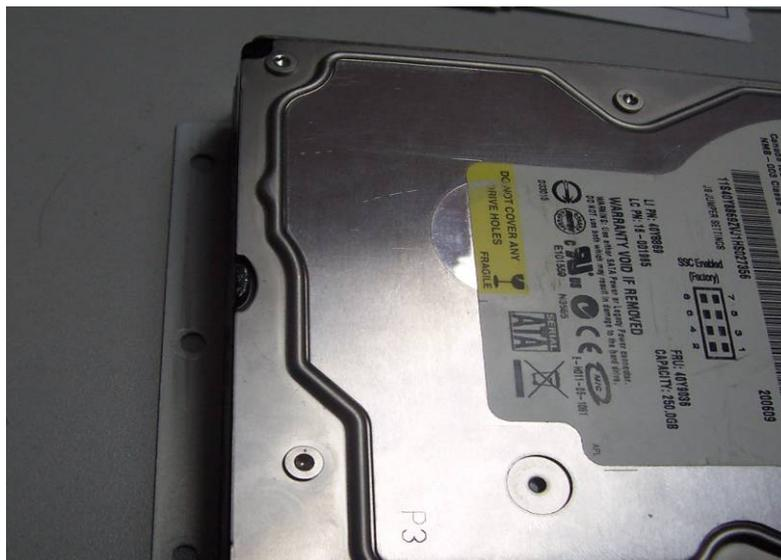
5) Fix the HDD plate on the DVR device and then cover the DVR and screw.
