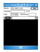
**STEP6** Input the server's address, ID and password respectively in the columns of "Server", "User" and "Password". And click "Go" to login the DVR. It will show the picture if access successfully.
