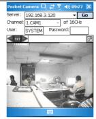
STEP7 Camera1 is the default display after login. Change the camera in rolling-down menu of "Channel".
